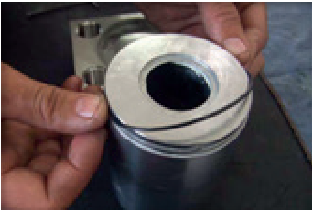
7° - Enter the O-Ring on tear shirt.
