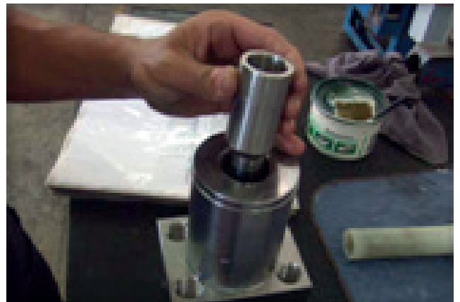
26° - Insert the bushing Support.
