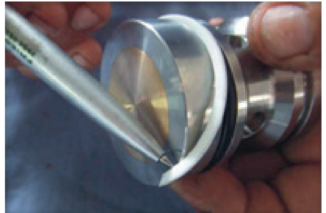
Put Bak ring, making sure that it is to the outside as well as the chamfer Bak Ring (indicated with the pen).
