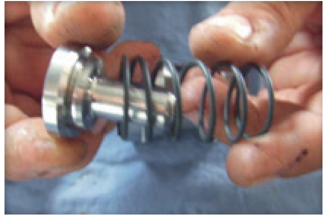
Fit the pressure spring (Pos. 15) in the Pressure Valve.
