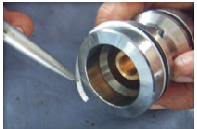
Perform the same process on the other hand, stressing attention on the chamfer bak ring.
