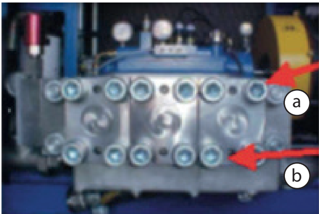
a) With the aid of a torque wrench, tighten the screws "X", with torque of 320 Nm. b) With the Assistance of an allen Wrench, pull the grub screws in "X".
