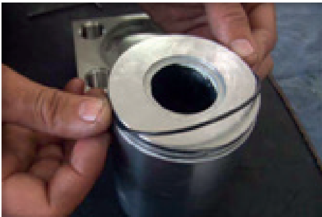
7° - Enter the O-Ring on tear shirt.
